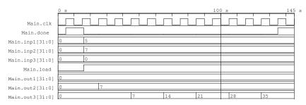
load is asserted at time 15 and done is T then, but done immediately drops to F in response to load being asserted. At the same time as load is asserted the
